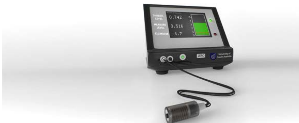
Magnetometer probe with a digital readout allows surgeons to accurately identify the sentinel lymph node in complex cancer types. Image by artist Nic Arrighi.
