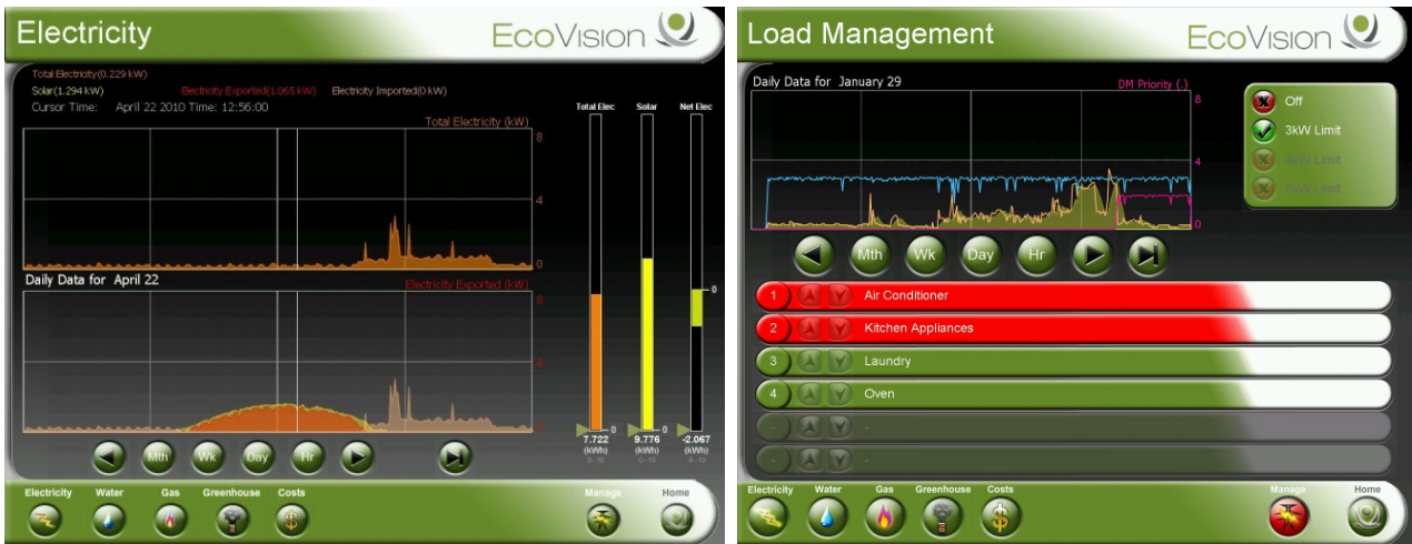
Figure 2: EcoVision screens, showing (a) electricity consumption and generation, and (b) appliances deactivated by the load management system, for a period of one day.
