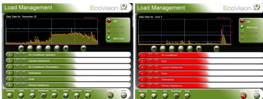
Figure 1: Load management system screens of two in-home displays for set points of (a) 5kW and (b) 3kW. Subfigure (b) highlights the power circuits that have had power interrupted.
