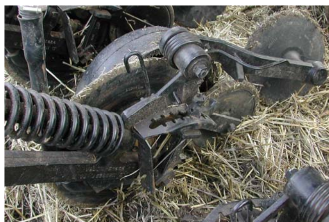
Low soil disturbance attributes of disc seeders were seen to minimise seedbed moisture loss, reduce weed pressure and improve crop establishment in marginal moisture conditions
