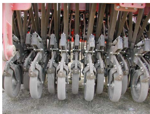
Disc seeders were cited as well suited to narrow row spacing requirements such as for pasture establishment and renovation
